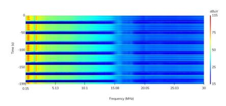
sweeps and can recover any of these slices for analysis and comparison purposes with, for instance, a standard limit. It can also be applied to common and differential-mode measurements.
